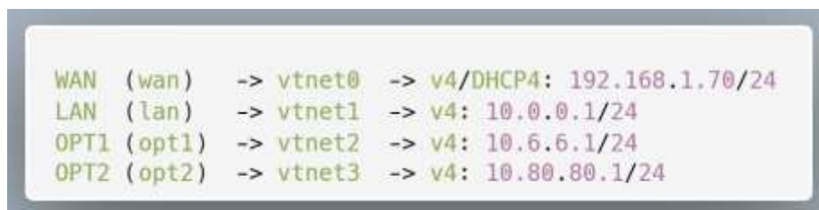
Figure 1 Final pfSense network configuration as seen from the console
